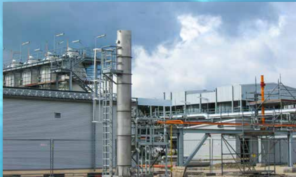
↑ Flashgas flare for RAG - 50 m 3 /h flash gas Underground gas reservoir 7 FIELDS in Austria
