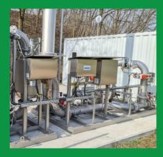
The temperature in the reactor shifts in the direction of flow so the direction is changed in a switch box depending on the temperature. The reactor thus acts as a recuperative heat exchanger.
